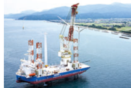
Offshore Construction Using a Self-Elevating Platform (SEP) Vessel
