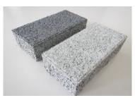
Interlocking block prototype
