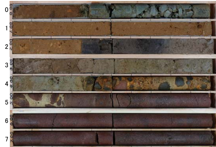
US-N07(孔口標高43.47m, 掘進長8m, 鉛直)
