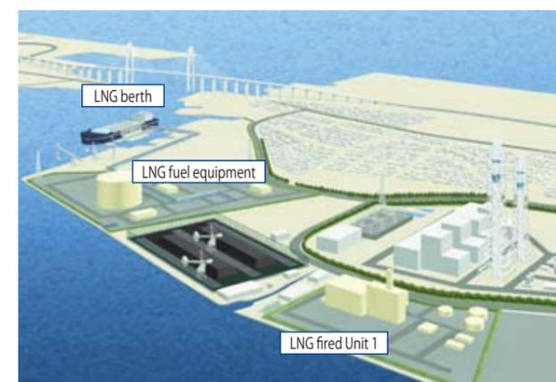
Image diagram of LNG fired Unit 1 of Toyama-Shinminato Thermal Power Station
