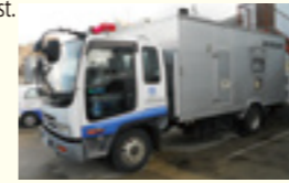
Power supply vehicle [specifications] 300 kVA x 5 vehicles
